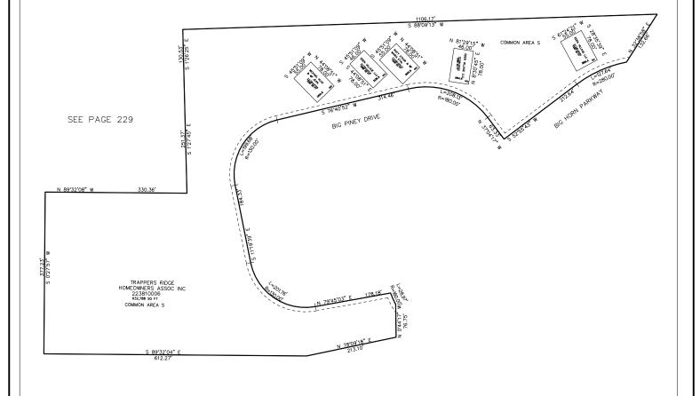
10' UTILITY & DRAINAGE EASEMENTS EACH SIDE OF PROPERTY LINES AS INDICATED BY DASHED LINES EXCEPT AS OTHERWISE SHOWN.
